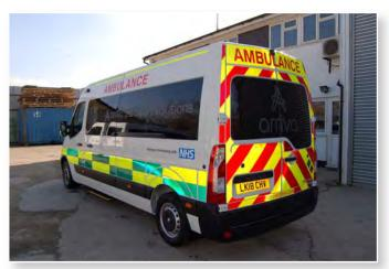
The Blue Light Services Multiplex PTS Vehicle is designed to allow the vehicle to be reconfigured on a daily basis to meet the changing needs of a NEPTS contract. The vehicle can change configuration from 6 seated, 2 wheelchairs & 4 seats or a stretcher & 4 seats in a matter of seconds due to the patented Mult plex sliding seat system.
